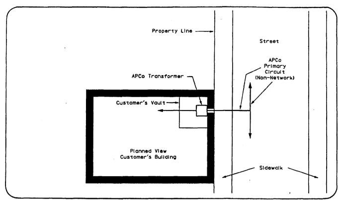
Designated Underground Area Building Set At Property Line Primary Underground to Transformer in Customer Vault Secondary Underground Service Secondary Metering
