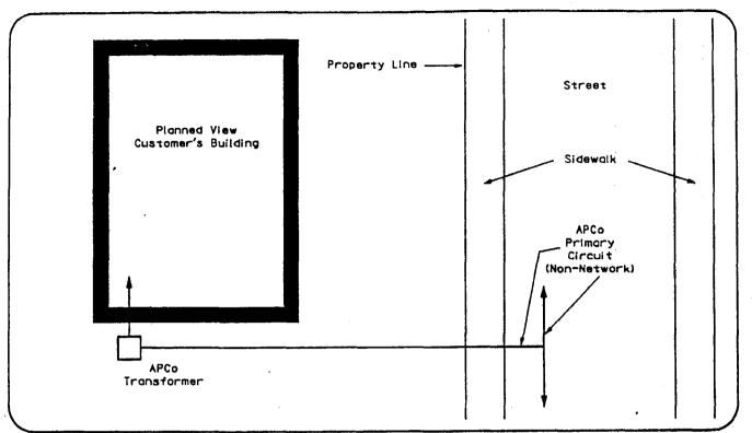
Designated Underground Area · Building Set Back From Property Line · Primary Underground to Transformer Located Outside of Building · Secondary Underground Service · Secondary Metering
